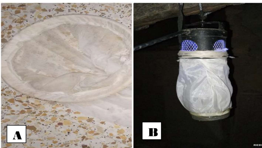
Figure1: Phlebotomine sand flies sampling Materiel: (A) sweet net & (B) CDC miniature light.
