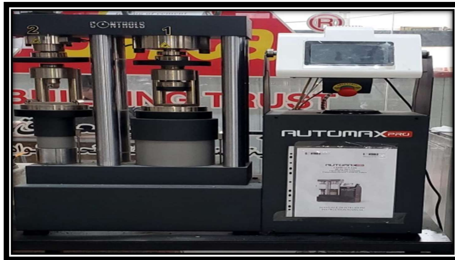
Figure (5): Compressive strength testing device
