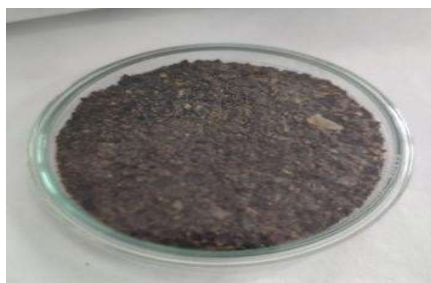
Figure 7: Jatropha curcas Seed waste as a substrate mixed with Saccharomyces cerevisiae
