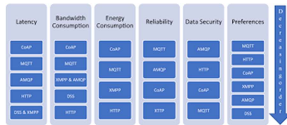
Fig. 2.2.1: Communication Protocols in Industrial Environments
