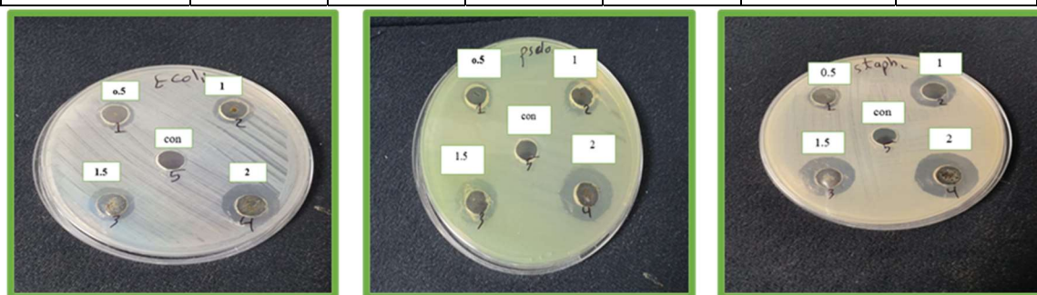
Figure (4) Antibacterial activity against E.coli , Pseudomonas aeruginosa and Staphylococcus aureus for different concentrations of silver nanoparticles manufactured using Spirulina platensis algae extract.
