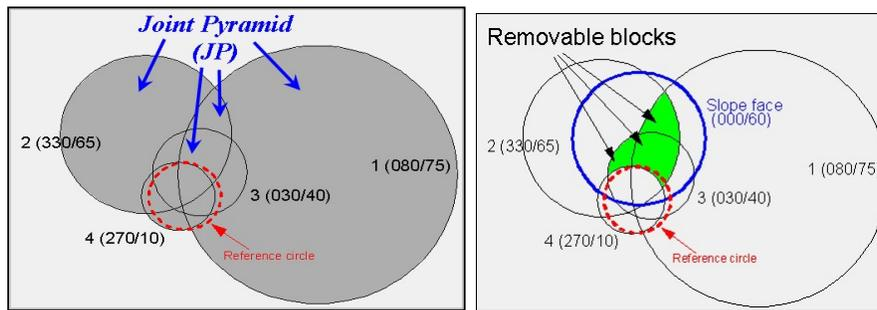
Figure 3. Identification of removable blocks on stereonet.
